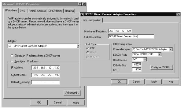
TCP/IP Direct Connect Configuration Screens Figure 5-26.
